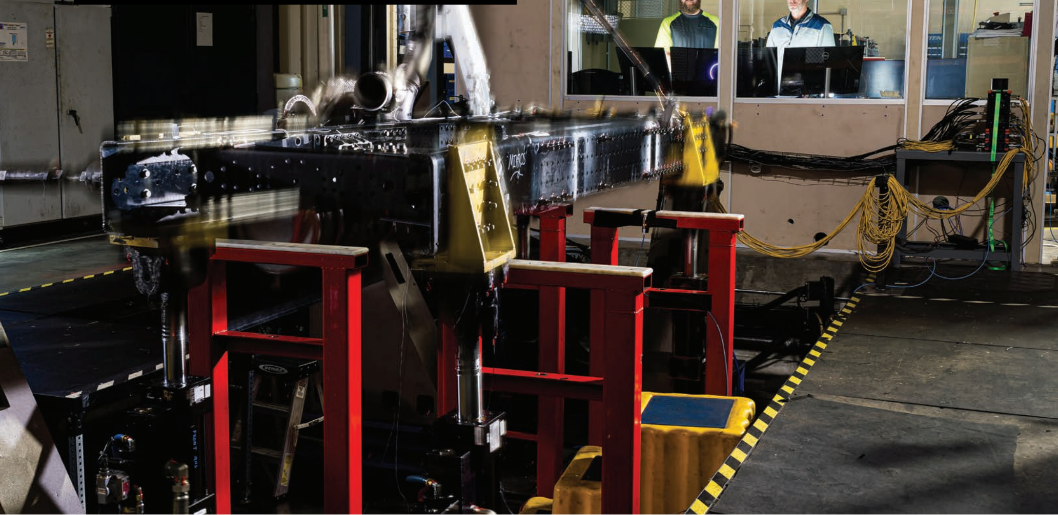
Jonathan Abernathy (left) and Evan Kimbro (right) control a chassis shaker test. The hydraulic actuators bolted to the frame subject it to repeated violent stresses.
